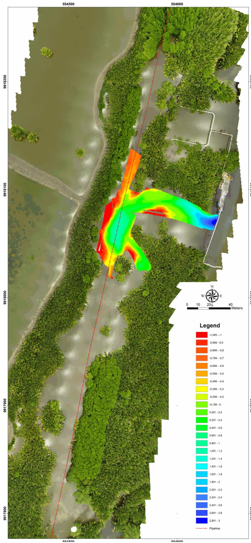
Figure 9. Depth contours from MBES data. The red dashed line is the pipeline position from database
