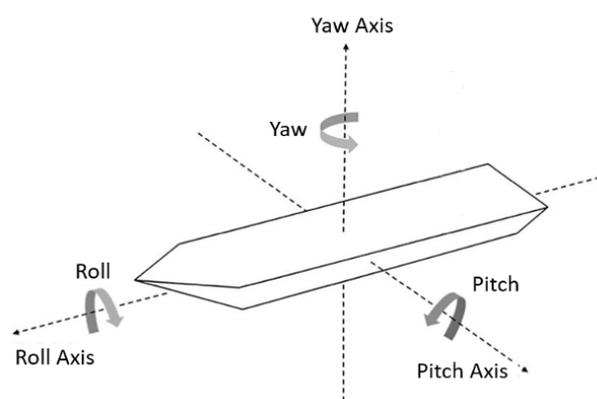
**Figure 4.** Illustration of USV's movement on water surface
