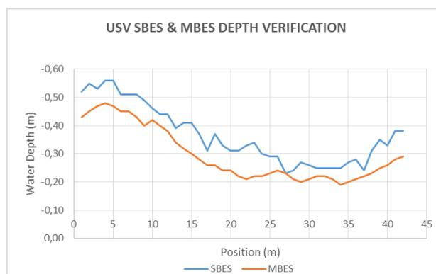
**Figure 5.** Depth profile from SBES (blue line) and MBES USV (red line) with a difference of 0.07 meter (average)
