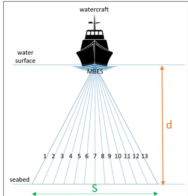
**Figure 1.** Illustration of sonar beams on bathymetric operation using Multibeam Echosounder (MBES). The MBES device attached at the keel of the watercraft releases 13 beams to the seabed and records the reflected beams from the seabed. S refers to swath width while d is the depth of water
