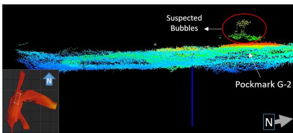
Figure 15. Suspected bubbles around G-1, G-2, G-3 location on day 2 (October 30, 2021) during MBES data processing
