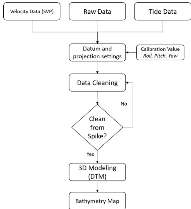
**Figure 7.** Bathymetry data processing flow chart
