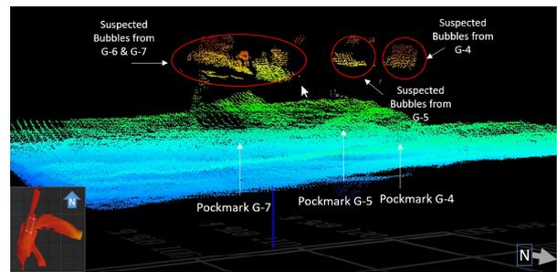
Figure 16. Suspected bubbles around G-4, G-5, G-6, G-7 location on day 2 (30 October 2021) during MBES data processing
