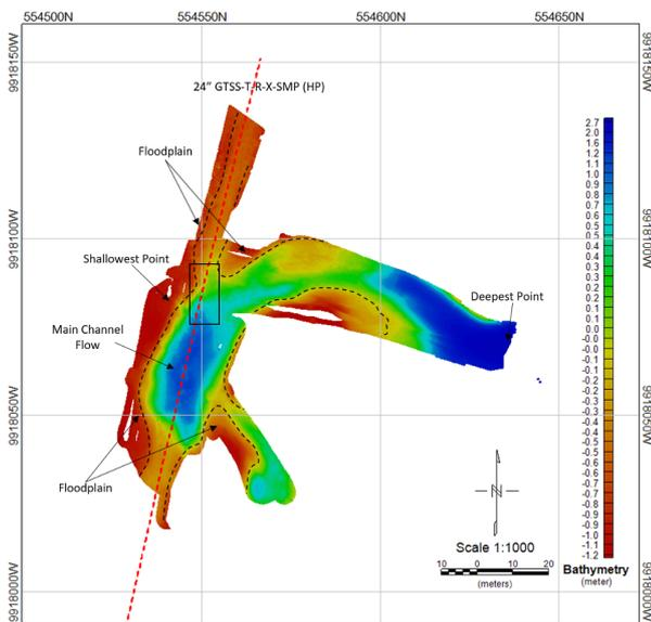
**Figure 10.** Multi beam bathymetric map of the 24 inches Pipeline USV survey area. The red dashed line is the pipeline's position from the database
