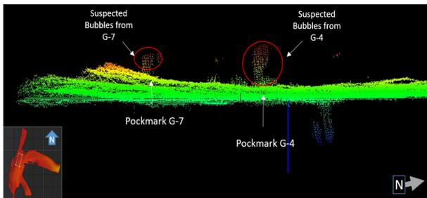
Figure 14. Suspected bubbles around G-4 and G-7 location on day 1 (October 29, 2021) during MBES data processing
