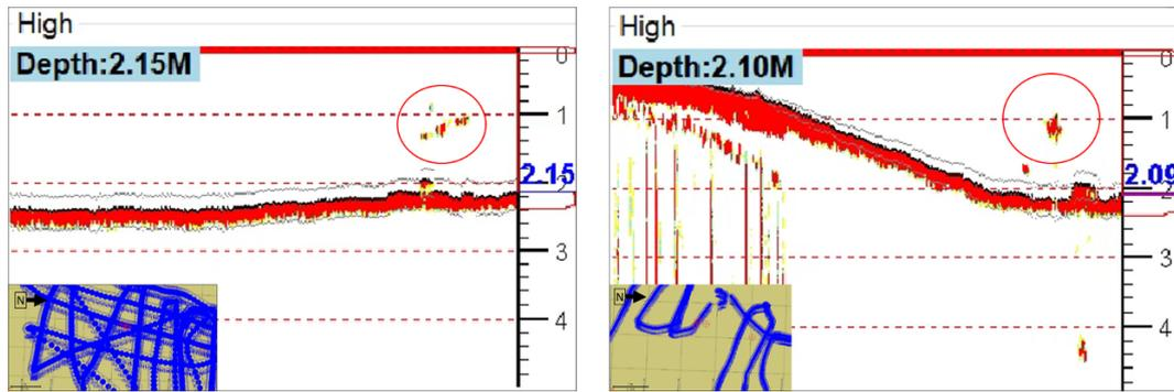
Figure 12. Suspected bubbles (red circle) at G-4 from SBES recorded data (left image is line track North to South and right image is line track West to East)
