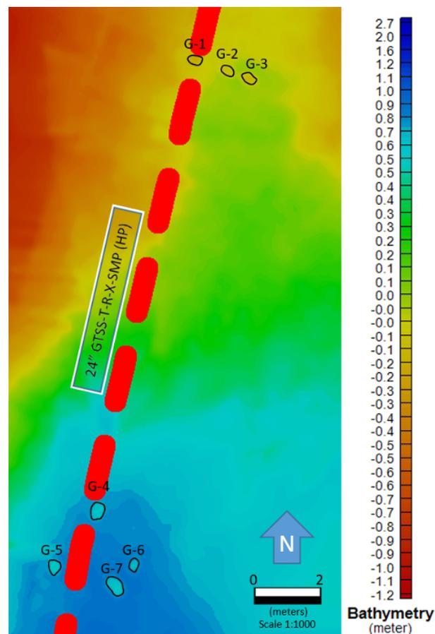
**Figure 11.** A zoomed in image of anomalies near the 24 inches pipeline area. The red dashed line is the pipeline's position from the database
