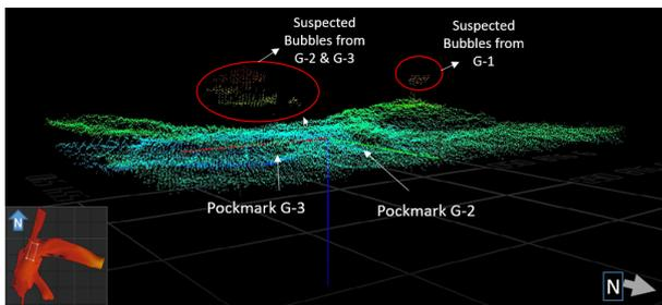
Figure 13. Suspected bubbles around G-1, G-2, G-3 location on day 1 (October 29, 2021) during MBES data processing
