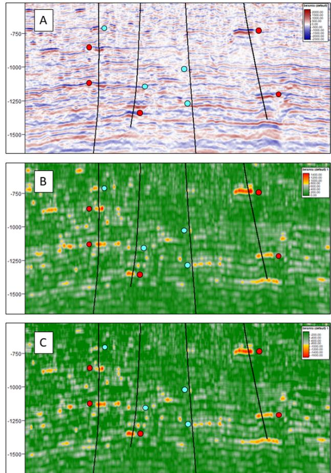
Figure 6. A) Seismic line from Shallow interval of Tunu field, crossing several wells. Black lines are the well trajectories. B) Intercept from Slope of Spectral Amplitude at the same line. C) Gradient from Slope of Spectral Amplitude at the same line. Red dots show where there is gas, blue dots show where there is no gas.
