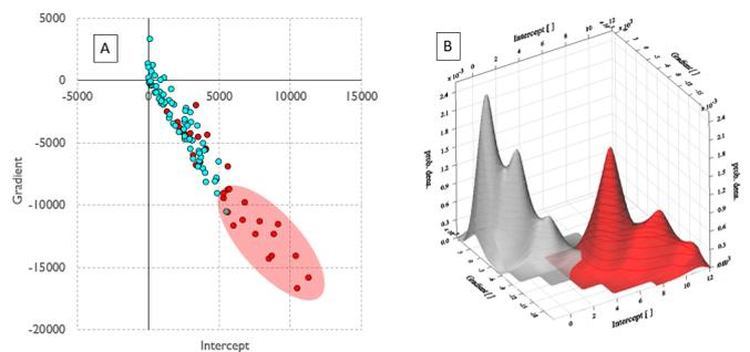
Figure 7. A) Cross plot between Intercept and Gradient at several well samples. Red dots represent gas samples; blue dots represent non-gas samples. Gas cluster is interpreted as red oval polygon. B) The simplified Probability Density Function (PDF) designed based on the Intercept and Gradient cross plot. Red surface represents the gas definition; grey surface represents the background (non-gas) definition.
