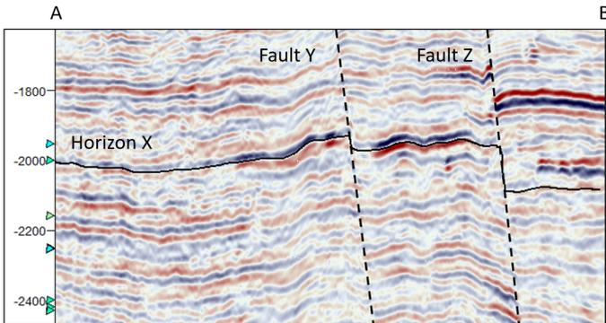
**Figure 8.** Seismic line from Fresh Water Sand interval of Sisi Nubi field, crossing two major faults. Bright amplitudes were observed at Horizon X location.
