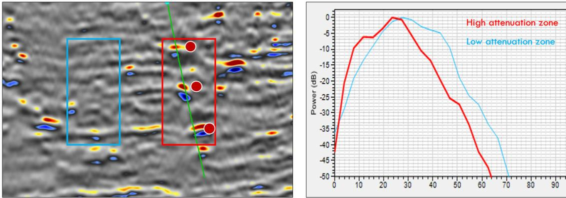
Figure 1. Seismic frequency spectrum differences (right) related to hydrocarbon and non-hydrocarbon presence (left).
