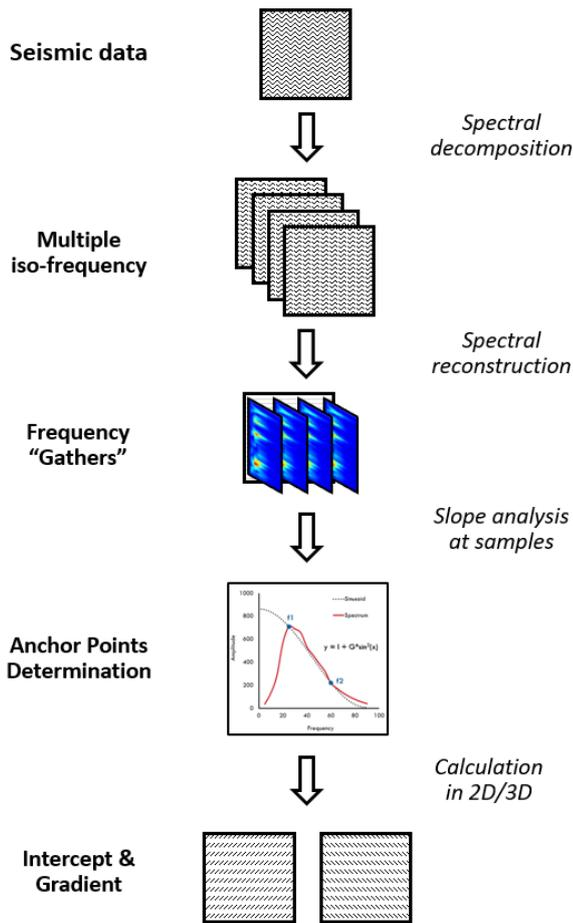
Figure 5. Slope of Spectral Amplitude workflow
