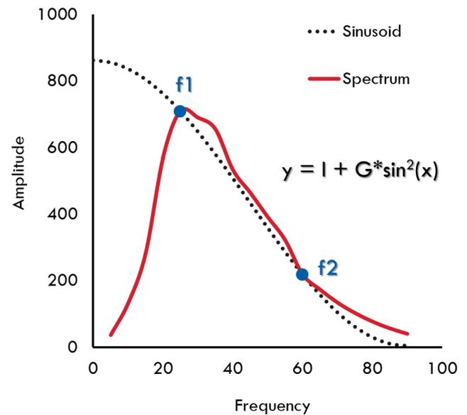
Figure 4. Intercept and Gradient estimation using quadratic sinusoidal function
