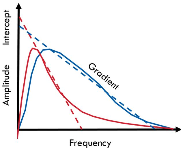
Figure 2. Attenuated seismic frequency spectrum characterized by Intercept and Gradient.
