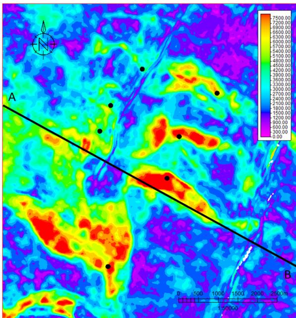
**Figure 9.** RMS amplitude map with 50ms window using Horizon X as reference. Black line shows the seismic line. Black dots represent gas found in wells.
