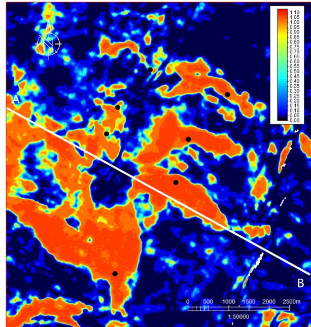
**Figure 10.** Gas Probability map with 50ms window using Horizon X as reference. White line shows the seismic line. Black dots represent gas found in wells.
