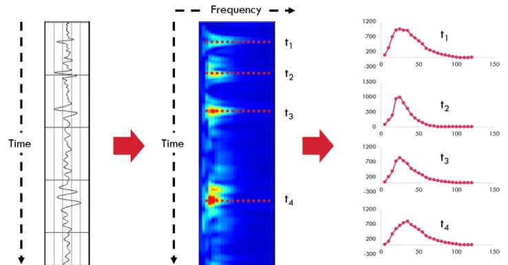
Figure 3. Spectral decomposition gives seismic spectrum details for every time samples
